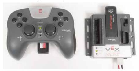
f. If the units fail to "Link Up", turn them both Off and back On. If they still fail to Link Up, tethering may be required. Refer to the section 1 for tethering instructions.
