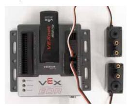
b. Motor Reversing: The Default Code allows jumpers or switches to be installed in the Digital Ports to invert the motor direction. This is useful to correct the direction of motors without changing code, or when using a switch to reverse a motor if the robot hits an object. The following picture shows motor reversing jumpers installed in Digital Ports 2 and 5 to reverse Motor Ports 2 and 5.
