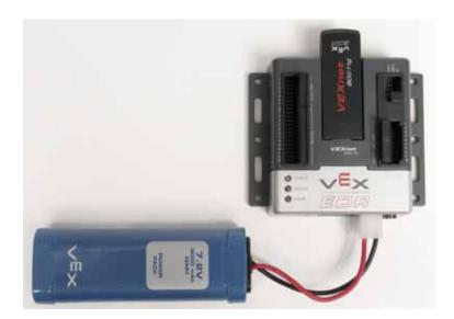
a. Attach 7.2v battery power and a VEXnet 802.11g key to the VEX CORTEX as shown.
