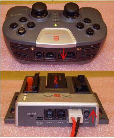
g. A valid link is as shown. The VEXnet light will be blinking a fast green on both units. The Robot light will wink green (be mostly on) on both units and when using fully charged batteries. It will take about 10 to 15 seconds for a link to be established. The Joystick light will be solid green when using fully charged batteries.
