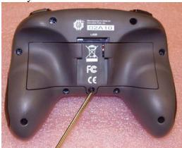
c. Install six identical batteries as shown. Use Alkaline, Ni-Cad or Ni-MH chemistries, but DO NOT mix different chemistry batteries. Charge rechargeable batteries only with a quality charger designed for your battery chemistry.
