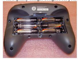
d. Reinstall the battery cover and add the VEXnet 802.11g key as shown. Insert the two tabs of the battery cover first along the back edge of the battery cover to aid in installation.
