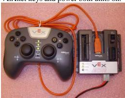
i. Add motors and test. The following picture shows 276-2163 motors plugged into motor port 2 and motor port 5. Pushing Joystick Channel 3 up will cause Motor 2 to turn clockwise. Pushing Joystick Channel 2 up will cause Motor 5 to turn counterclockwise.
