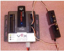
j. Motor Reversing: The default code allows jumpers or switches to be installed in the Digital ports to invert the motor direction. This is useful to correct the direction of motors without changing code, or when using a switch to reverse a motor if the robot hits an object. The following picture shows motor reversing jumpers installed in Digital ports 2 and 5 to reverse Motor Ports 2 and 5.
